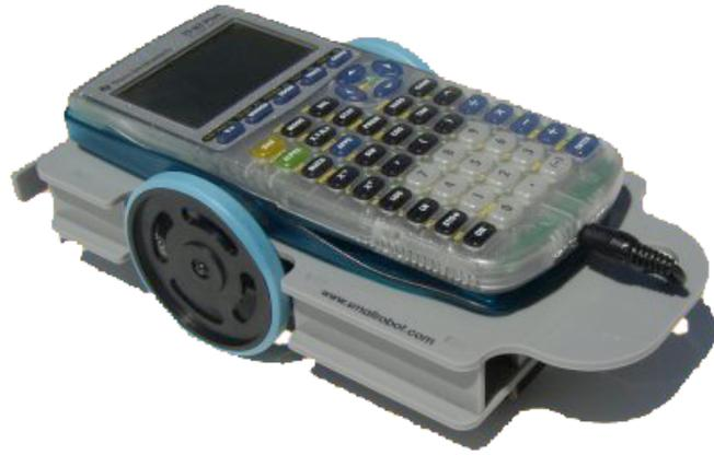
The directions for programming the robot claim that the duration values equate approximately to centiseconds. This can fluctuate due to environmental factors. We will complete an experiment to relate this number to angle turns in degrees.
